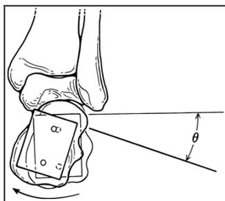
Figs. 3-A, 3-B, and 3-C: Illustrations showing how the gravity-dependent protractor was used to measure movement of the calcaneus at the subtalar joint. Fig. 3-A: To measure varus-valgus motion in the coronal plane, the protractor was placed on the superior surface of the aluminum block while the subtalar joint was maximally inverted and everted.  $\theta$  = varus-valgus arc of subtalar motion in the coronal plane.
