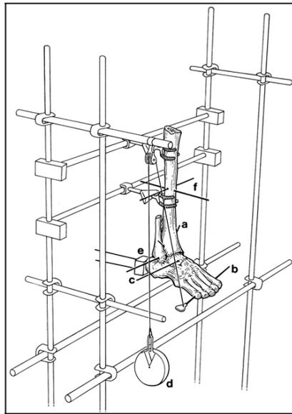
Illustration of the specimen in the frame. a = the Steinmann pins immobilizing the ankle joint, b = the Steinmann pin in the metatarsals, c = the Kirschner wires in the talar body and neck, d = the weight attached to the transmetatarsal pin, e = the aluminum block secured to the posterior aspect of the calcaneus, and f = the Steinmann pins in the tibial diaphysis that were used as reference points.
